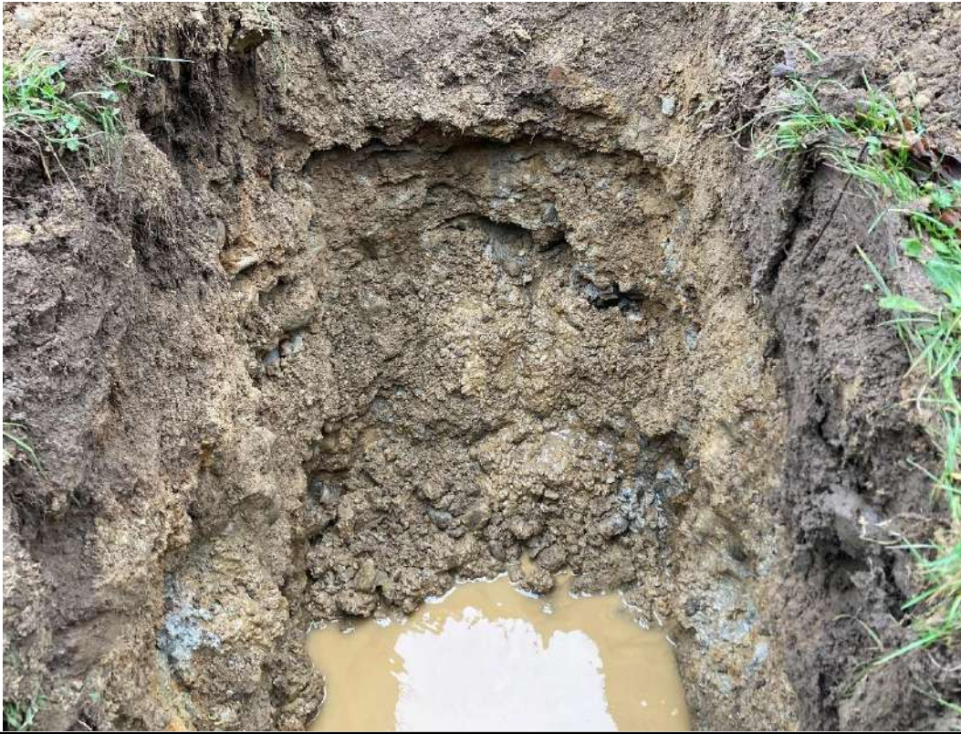
Plate 67 Groundwater encountered within TP06 once pit had been extended
