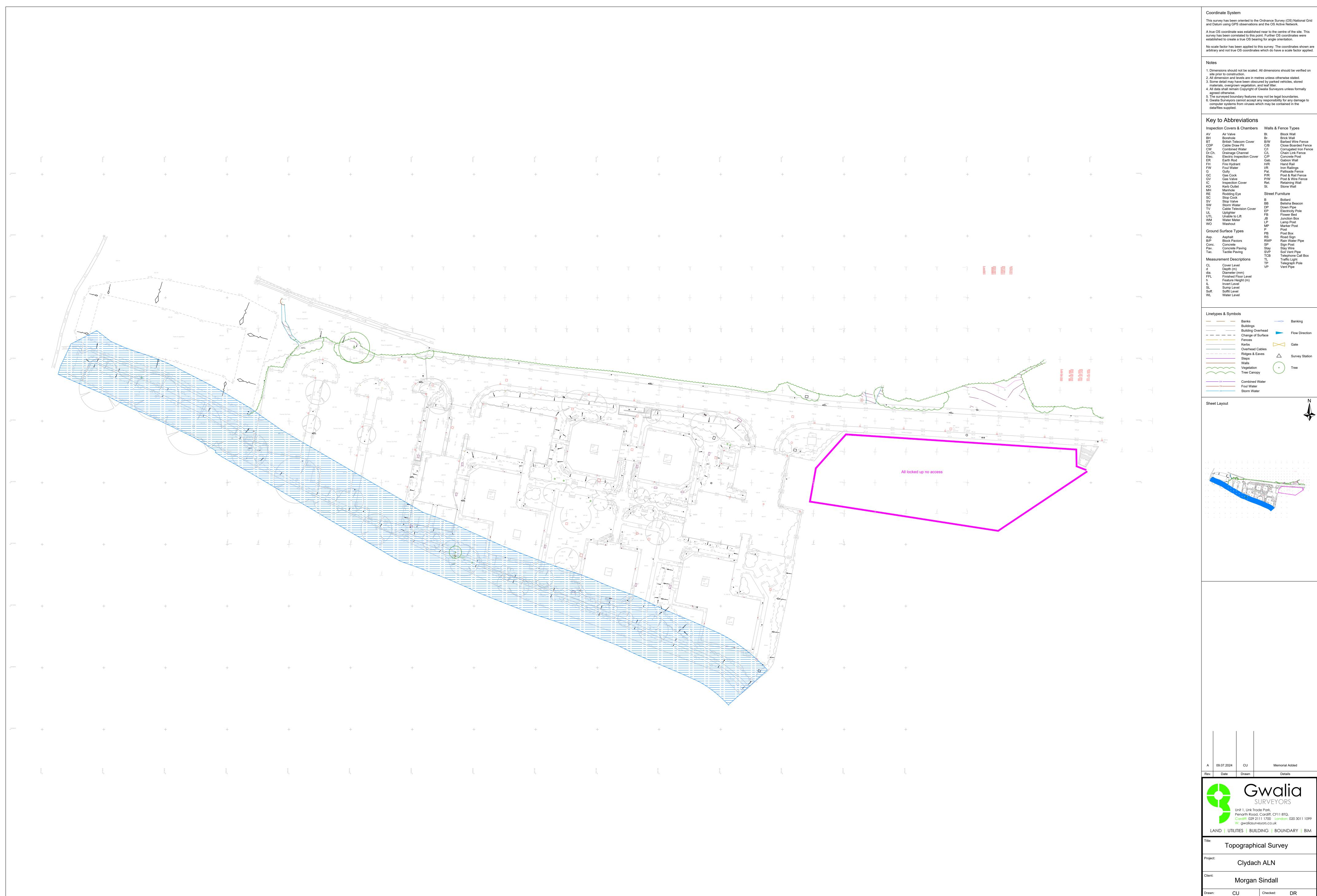
This survey has been oriented to the Ordnance Survey (OS) National Grid and Datum using GPS observations and the OS Active Network. A true OS coordinate was established near to the centre of the site. This survey has been correlated to this point. Further OS coordinates were established to create a true OS bearing for angle orientation.
