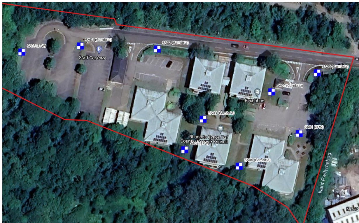
Figure 1 Soakaway Test Locations
