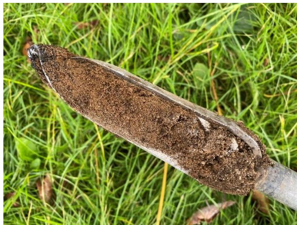
Plate 8: Auger arisings (TH9), showing intermixed material and fragments of foreign matter within Made Ground
