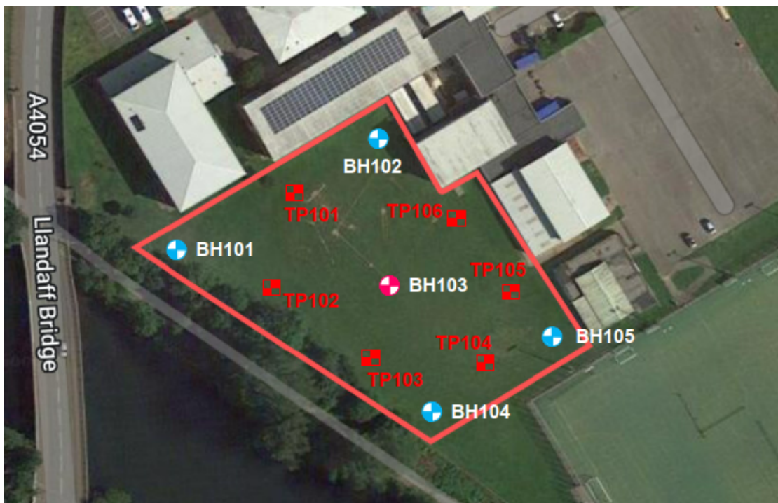
Fig 3.2 Soakaway test locations
