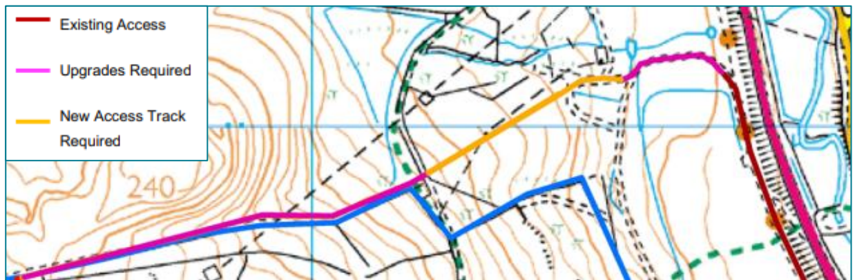
Figure 3.2: Approved plan of new and upgraded tracks
