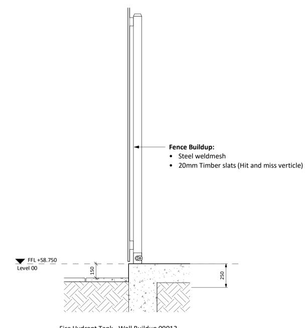
Fire Hydrant Tank - Wall Buildup 09012
