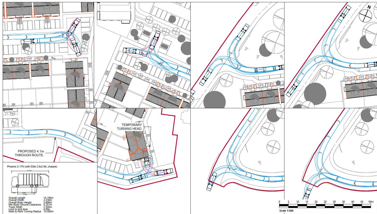
Figure 4-4: 10.2m Refuse Vehicle Swept Path Analysis
