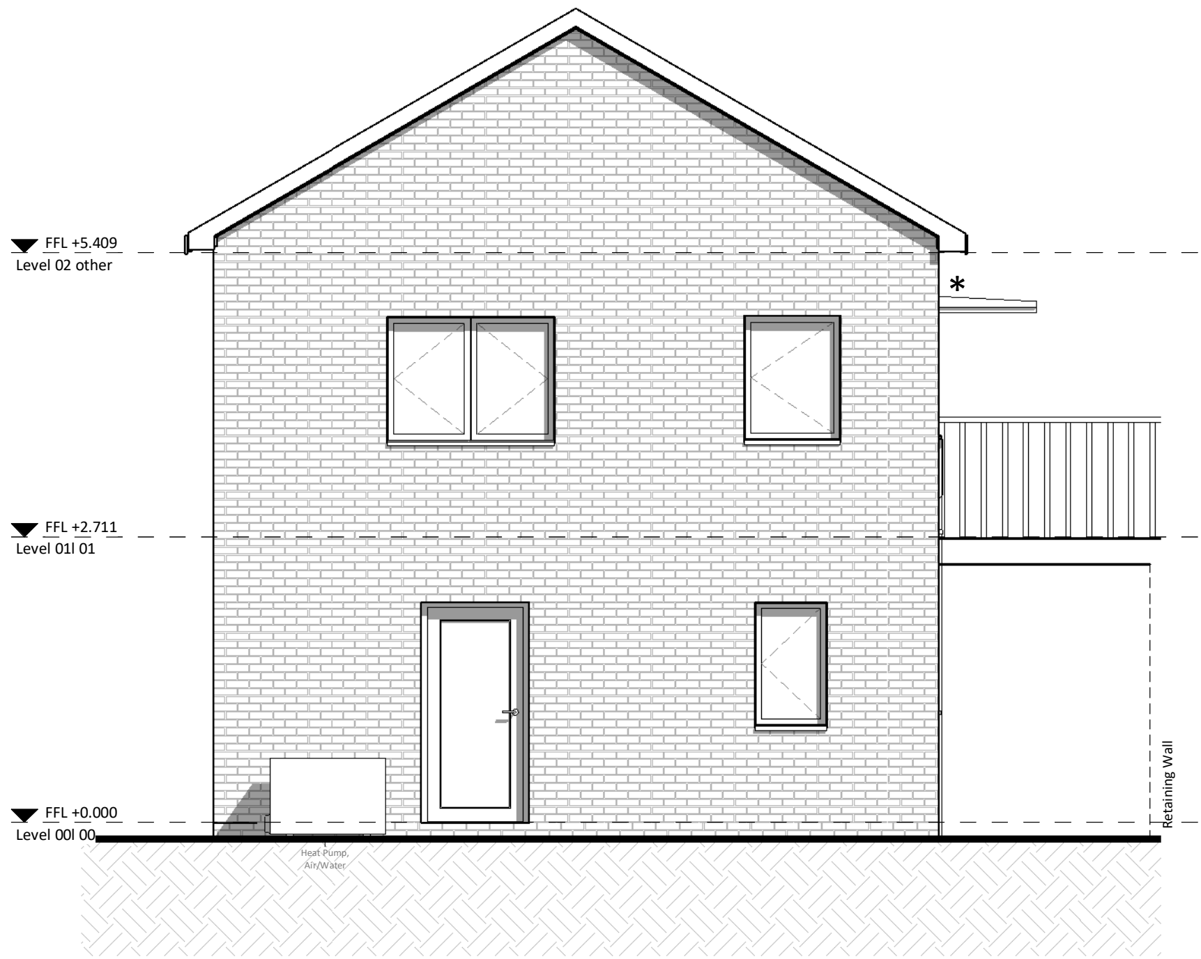
GA West Elevation 1 : 50
