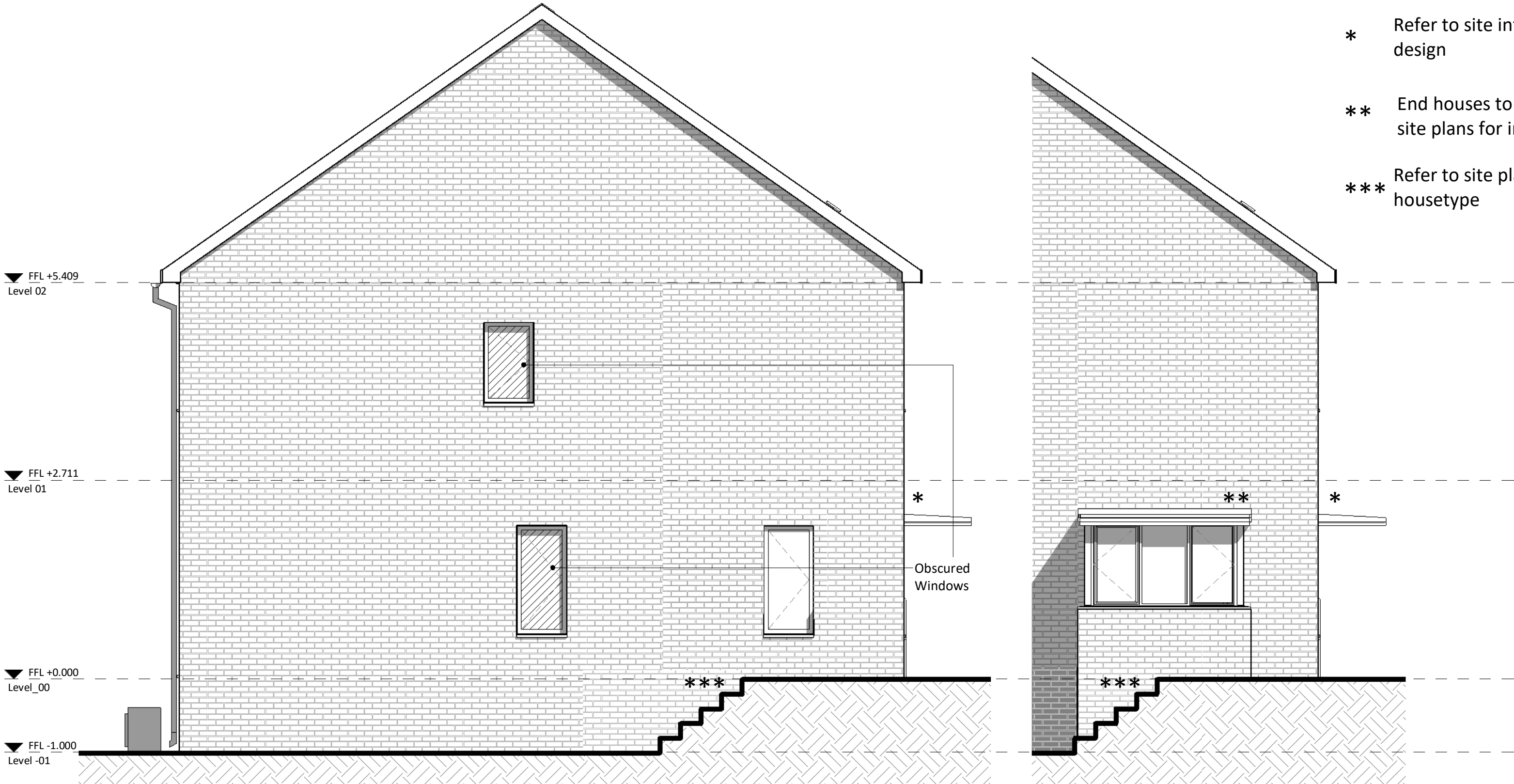
GA West Elevation 1 : 50
